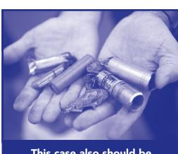
This case also should be a warning to all that lithium batteries can – and do – explode and can cause serious injuries.
